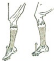
Saddle position should be such that the leg need never be straightened when pedalling.
