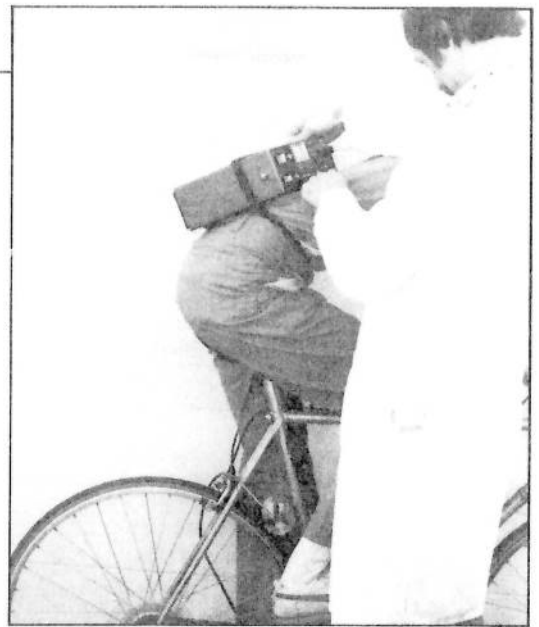
Figure 1: Four-channel cassette data recorder and tach-generator pickup by rider's leg. Marc Cole of Honda taking data.
