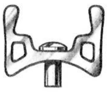
Inward-Slanted Sides-not a true hook-edge (Weinmann A129 concave)
