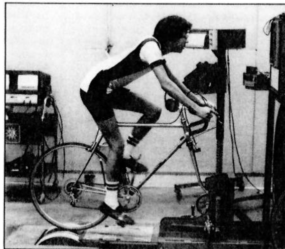
Figure 2: Honda's motorcycle dynamometer/simulator being used to measure power on Brian Uchida.
